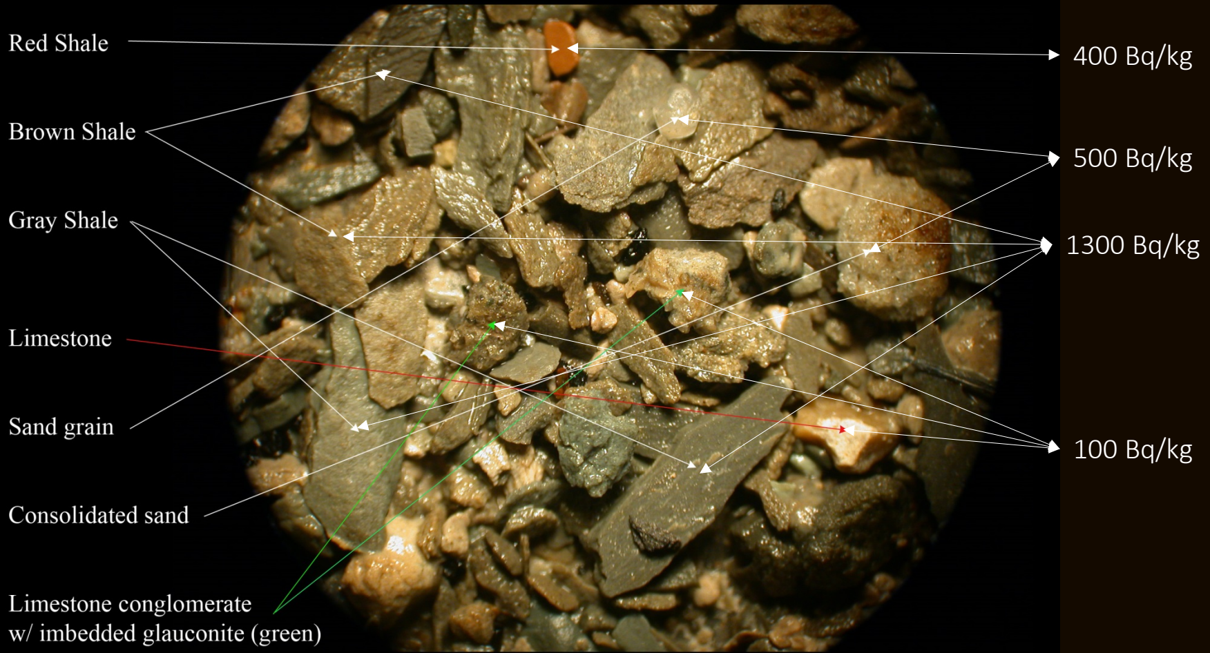
Sample of drill cuttings under a 10x microscope
